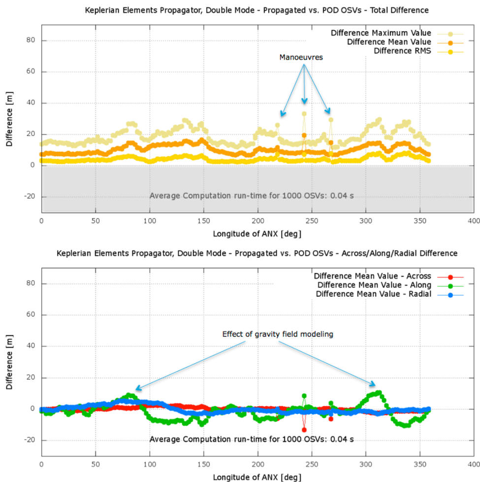
Figure 7 - Double mode propagator: difference as function of ANX longitude
