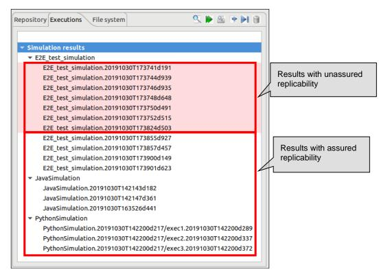
Figure 3-2: Executions tab and color code based on results replicability
