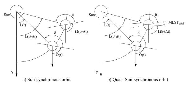
Figure 10: Sun-synchronous and quasi Sun-synchronous orbits descriptions
