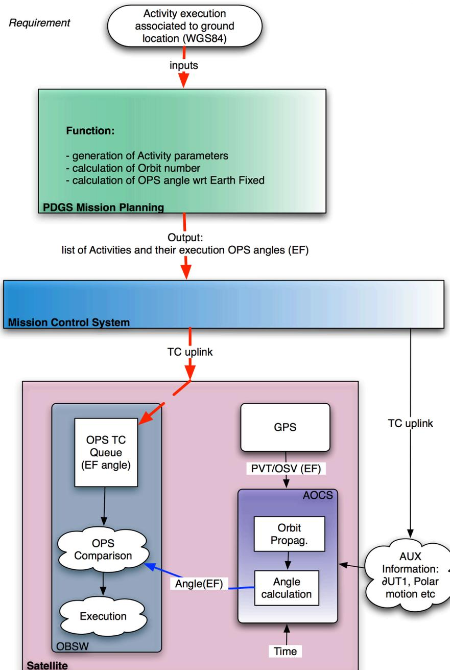
Fig 3. OPS angle end-to-end flow
