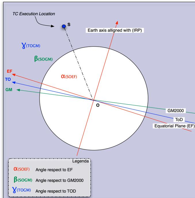
Fig. 1 OPS angle geometry shown in the GM2000 orbital plane.
