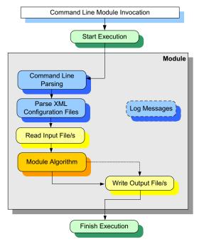
Figure 2-2: Normal Module Execution Flow Diagram
