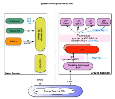
Fig 3. Ideal dataflow in ESA EO Ground System
