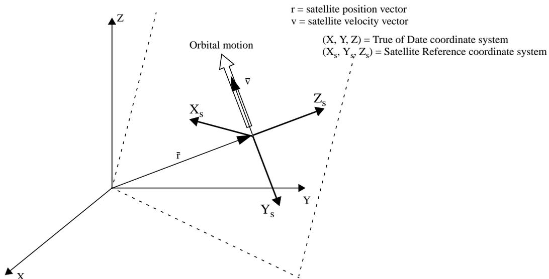
**Figure 3: Satellite Reference coordinate system**
