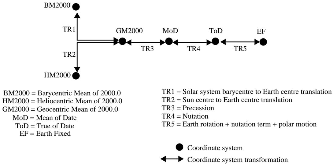
**Figure 5: Coordinate system transformations**
