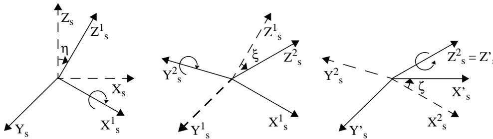
**Figure 4: Satellite Relative Reference coordinate system**
