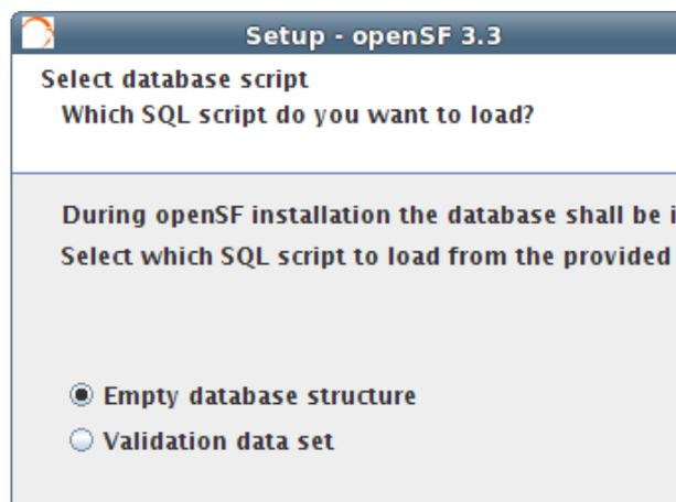
**Figure 3-7: Database structure selection dialog**
