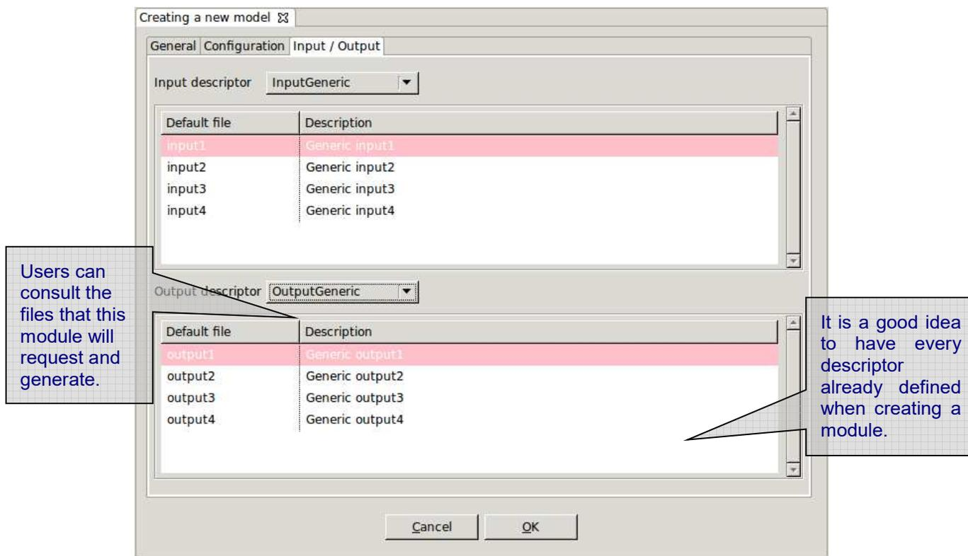
Figure 4-48: Module. Input/Output specification
