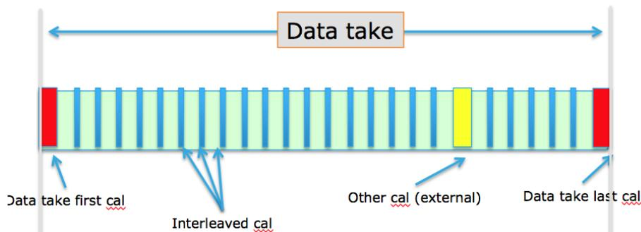
Figure 4-141 Example instrument operational mode scenario
