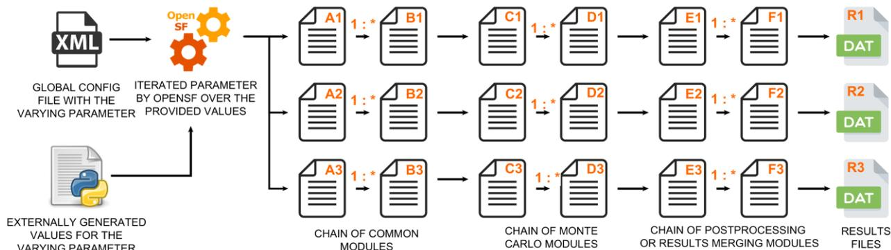
**Figure 4-140 MC with a global parameter**
