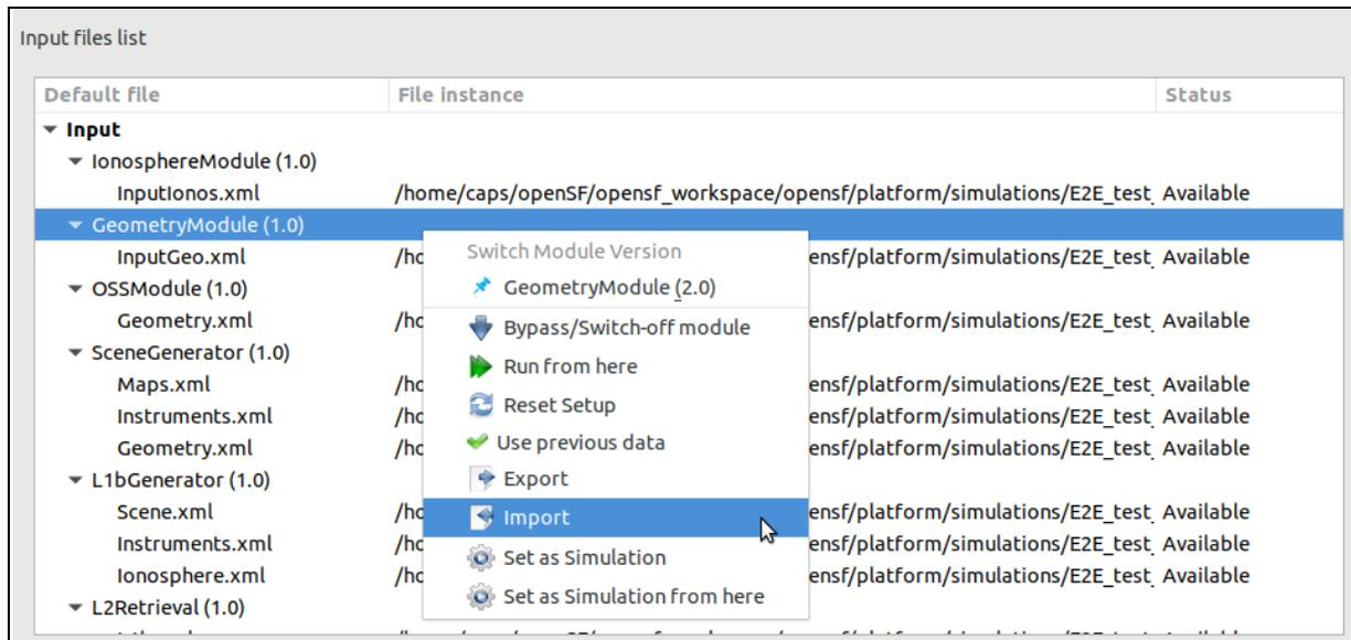
**Figure 4-94: Import module from the Simulation edition view**
