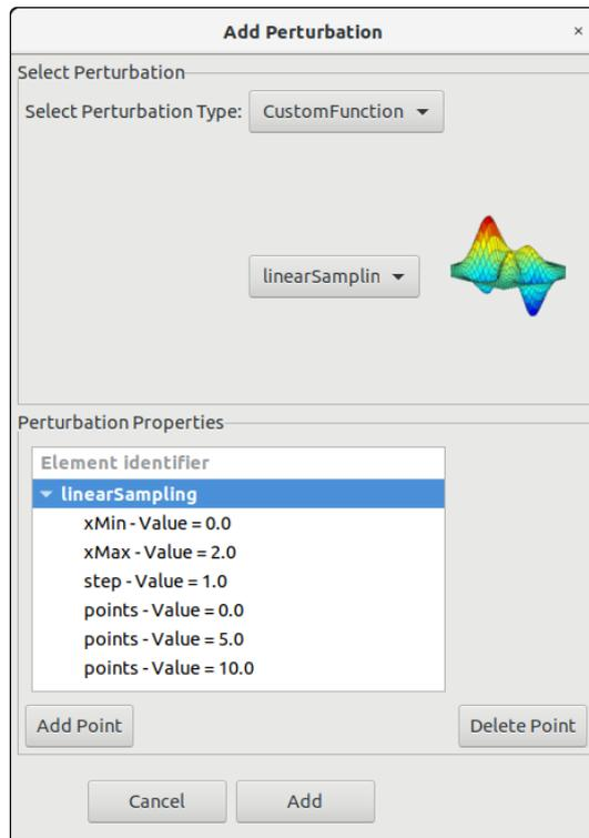
Figure 4-123 Function with variable number of properties (points)
