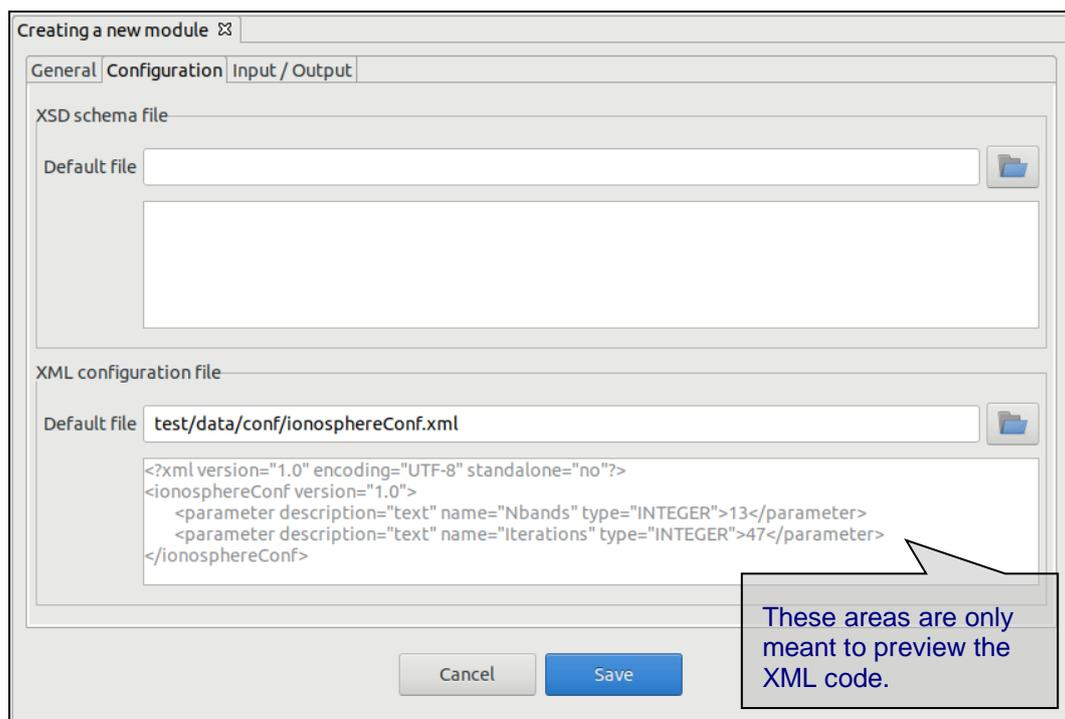
**Figure 4-47: Module. Configuration**
