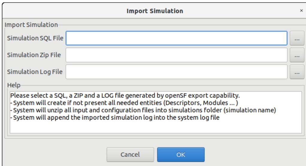
**Figure 4-91: Inputs requested for the import**
