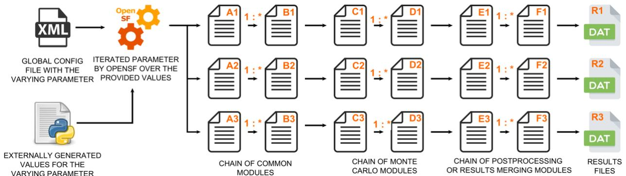
**Figure 4-131 MC with a global parameter**
