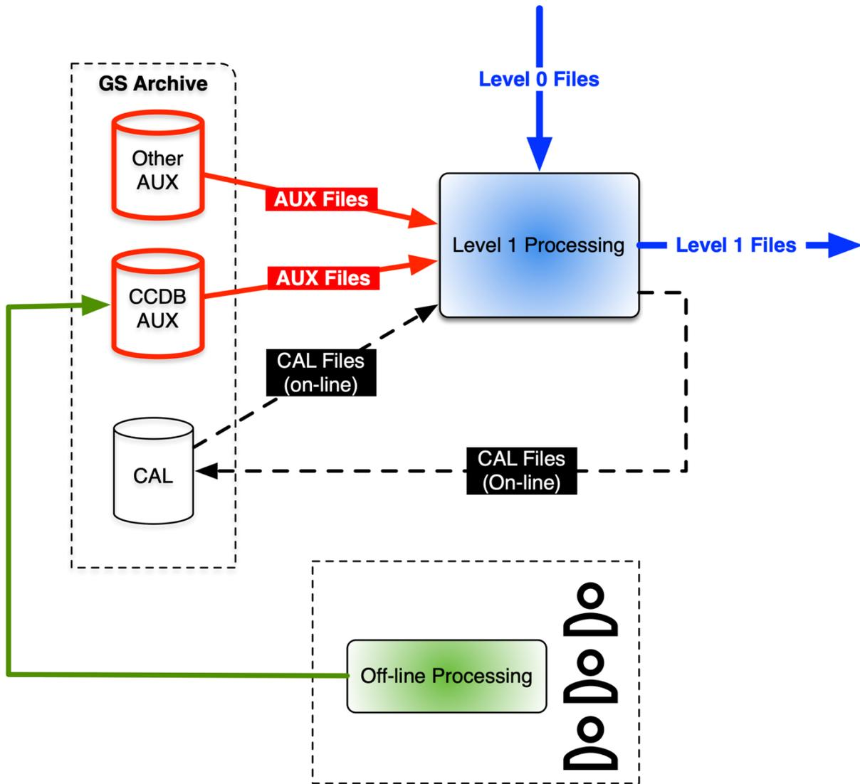
Fig. 1 Reference Data flow of AUX and CCDB related files
