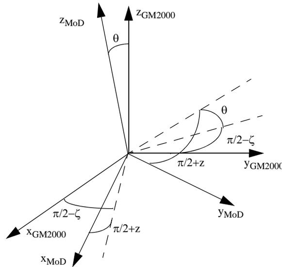
Figure 6: Transformation between GM200 and MoD reference frames
