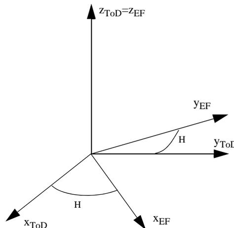
Figure 8: Transformation between ToD and EF reference frames
