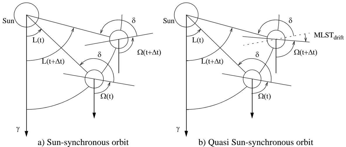
Figure 10: Sun-synchronous and quasi Sun-synchronous orbits descriptions
