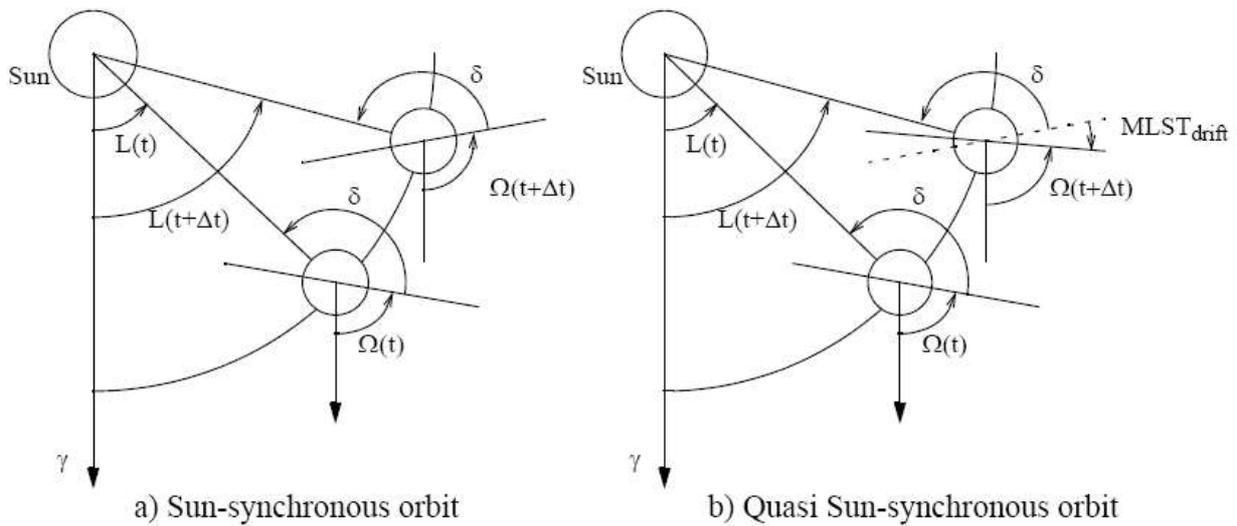
**Figure 11: Sun-synchronous and quasi Sun-synchronous orbits descriptions**
