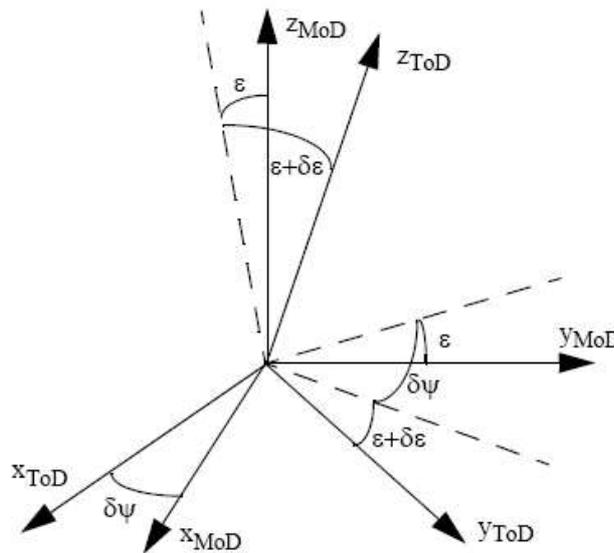
**Figure 7: Transformation between MoD and ToD reference frames**
