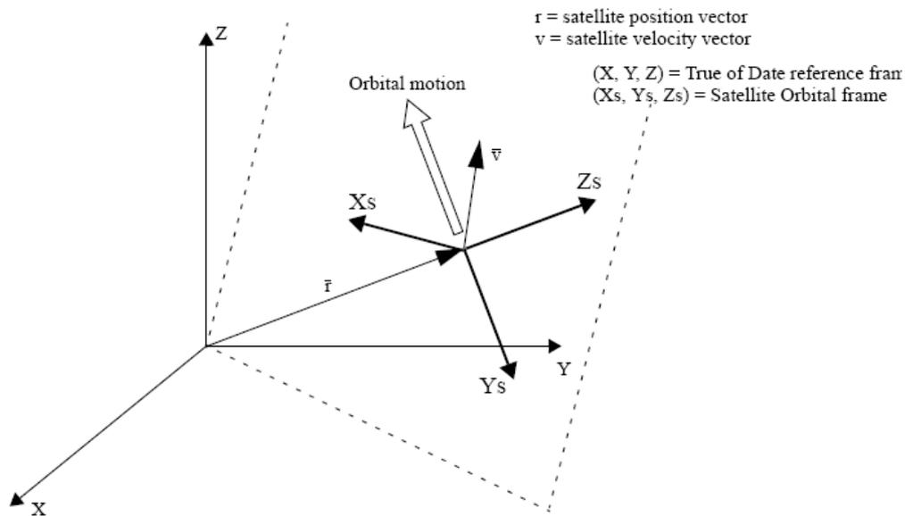
**Figure 2: Satellite Orbital Frame**
