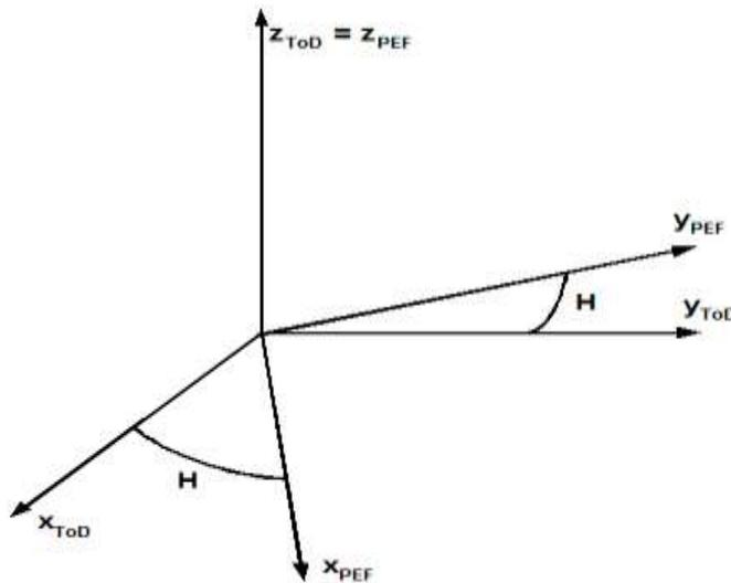
**Figure 8: Transformation between ToD and PEF reference frames**
