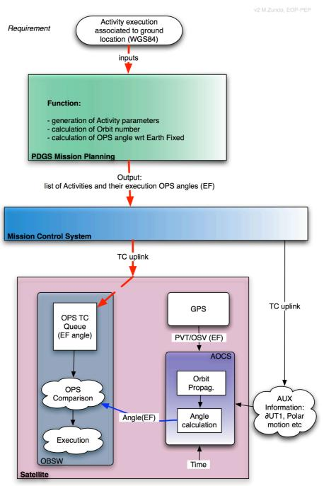
Fig 3. OPS angle end-to-end flow
