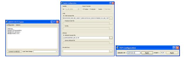
The <Satellite> <ID> shows the list of satellites defined in the current mission.xml file. The user selects the satellite to be driven.
