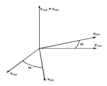
Figure 8: Transformation between ToD and PEF reference frames
