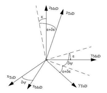
Figure 7: Transformation between MoD and ToD reference frames
