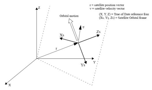
Figure 2: Satellite Orbital Frame
