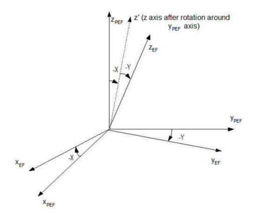
Figure 9: Transformation between PEF and EF reference frames
