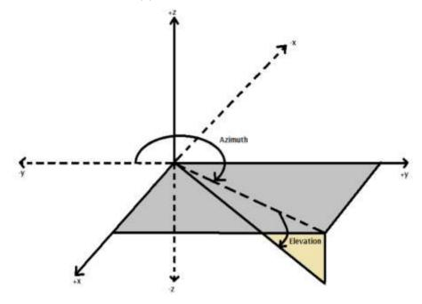
Figure 12: Azimuth and elevation definition
