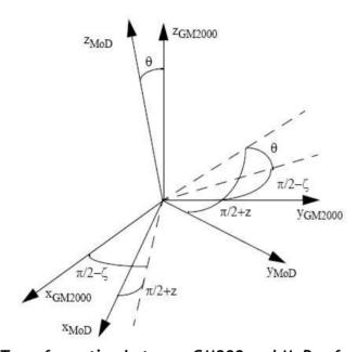
Figure 6: Transformation between GM200 and MoD reference frames
