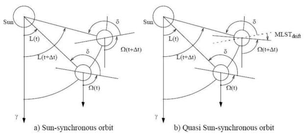
Figure 11: Sun-synchronous and quasi Sun-synchronous orbits descriptions
