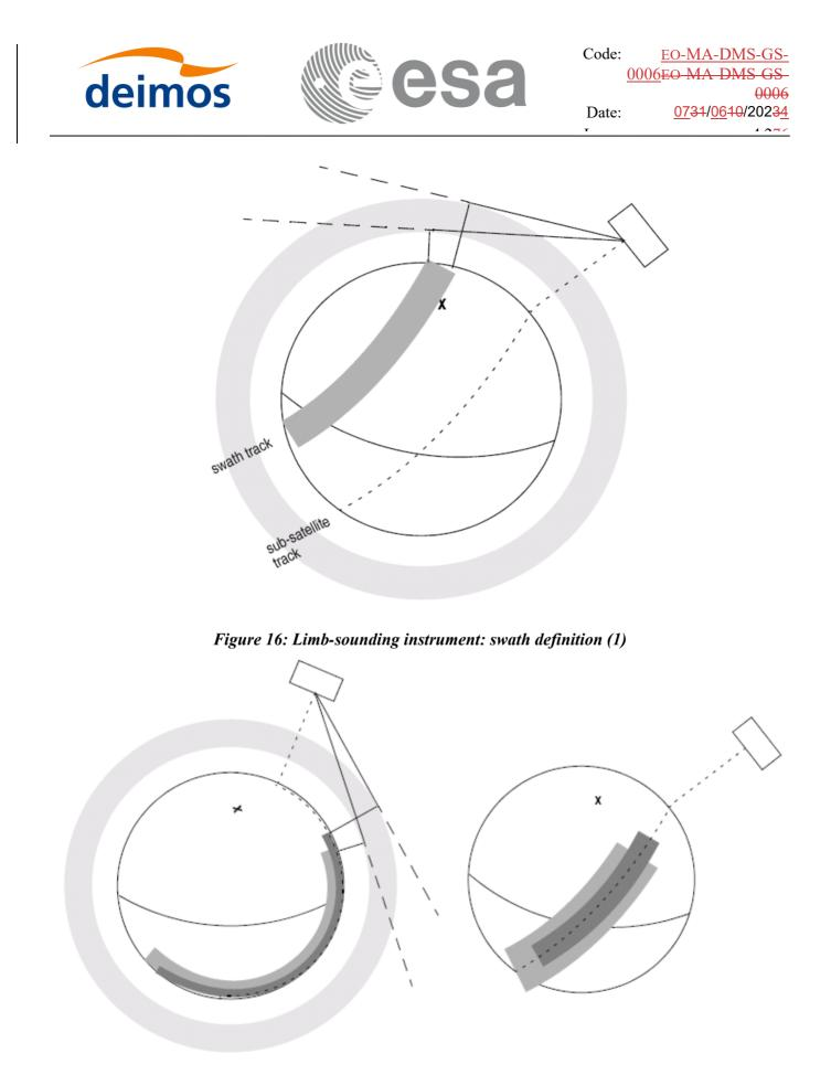
Figure 17: Limb-sounding instrument: swath definition (2)
