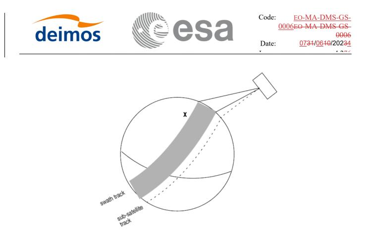
Figure 15: Earth-observing instrument: swath definition
