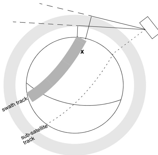
**Figure 5 Limb-sounding instrument: swath definition (2)**
