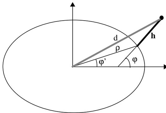
**Figure 7: Geodetic position**
