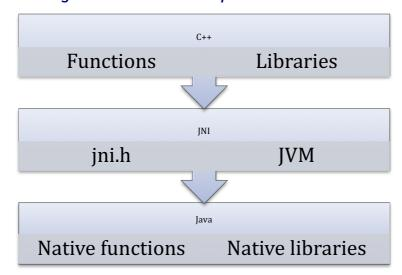
Figure 1 - C++ to Java top-level architecture
