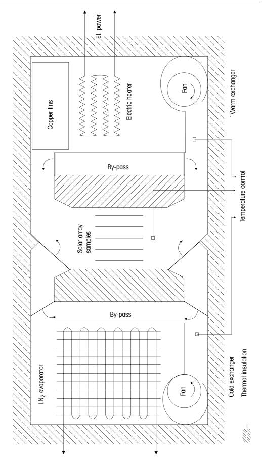
Figure 8: Accelerated thermal cycling test set-up
