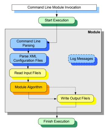
Figure 2-2: Normal Module Execution Flow Diagram
