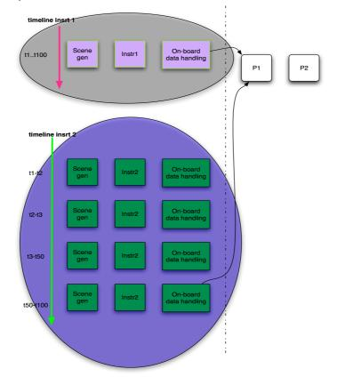
Figure 3-3 - Multi-Instrument E2E simulation with different timelines for each instrument
