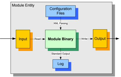
Figure 2-1: Module Entity Interfaces
