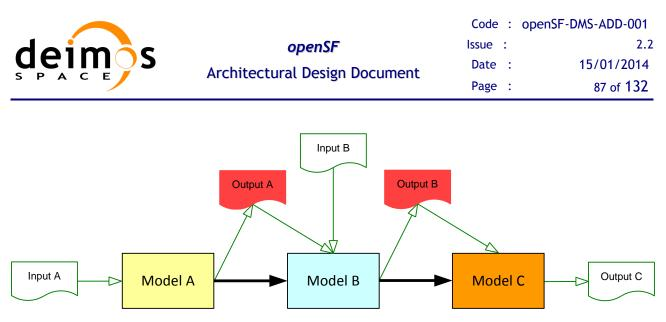
Figure 5-26: Removing intermediate data of a simulation
