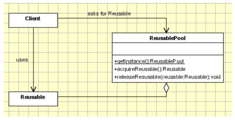
Figure 3-6 Thread Pool pattern example
