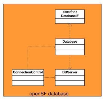
Figure 5-12: openSF.database class diagram
