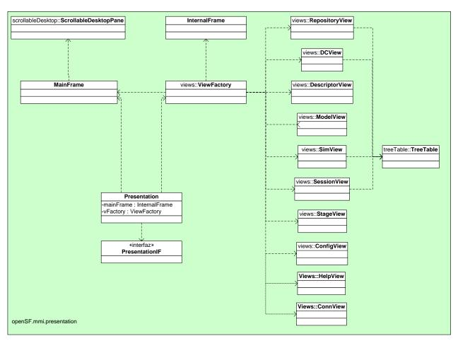
Figure 5-5: openSF.mmi.presentation package class diagram
