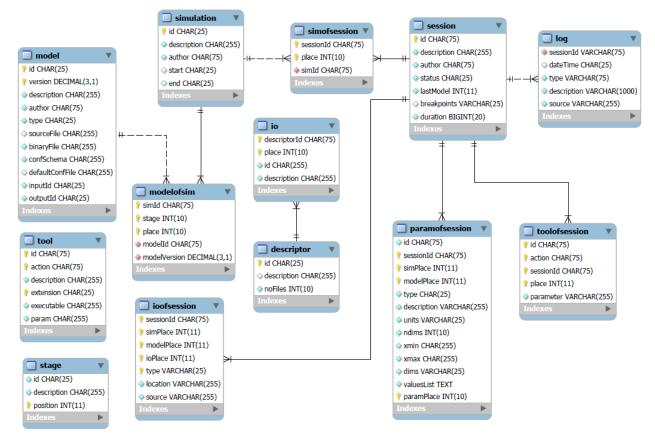
Figure 5-13: Database diagram<sup>1</sup>
