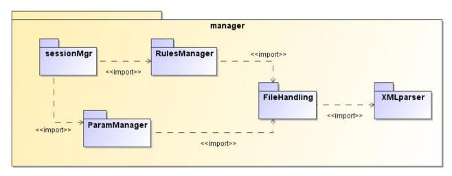
Figure 6-6: openSFpms.manager packages diagram
