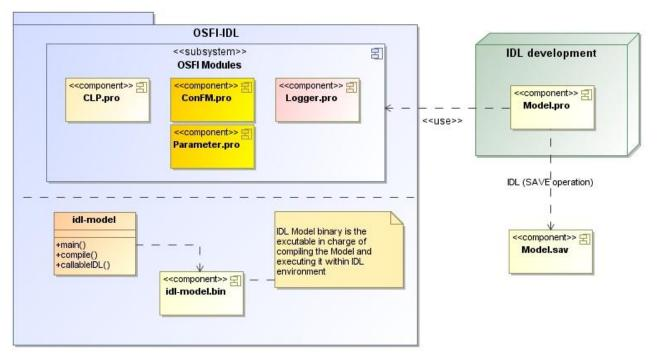
Figure 7-9: OSFI IDL implementation diagram
