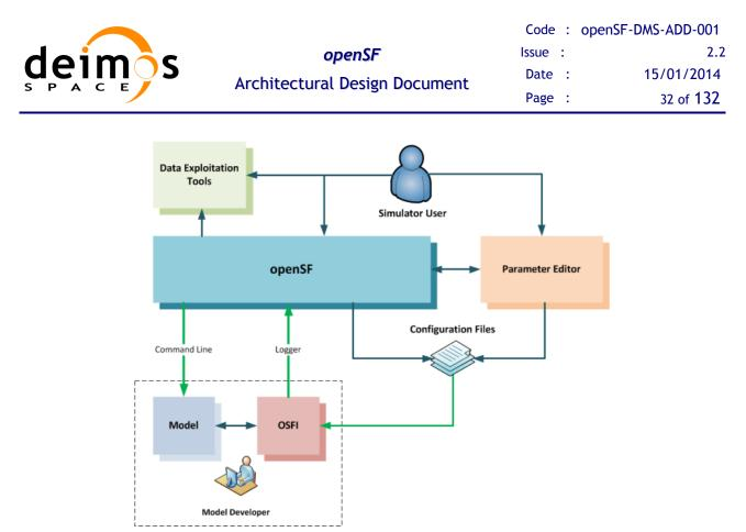
Figure 4-1: openSF High Level Architecture
