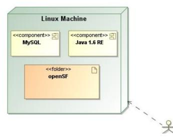
Figure 4-7 OpenSF deployment diagram
