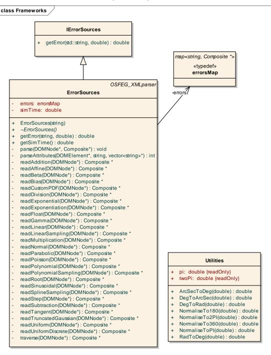
Figure 8-3: ErrorSources class diagram
