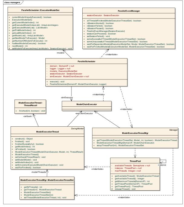
Figure 5-15: ModelChainExecutor class hierarchy for parallel model execution
