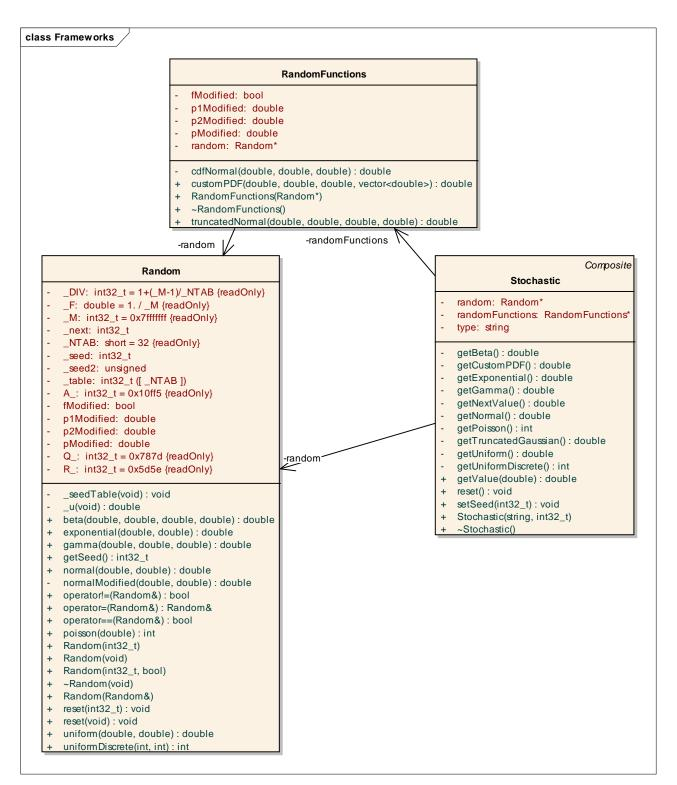
Figure 8-5: RandomFunctions hierarchy class diagram
