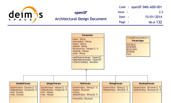
Figure 6-4: openSFpms.parameter class diagram
