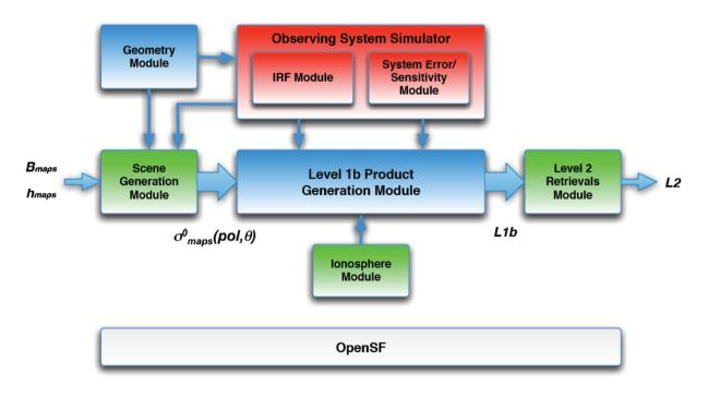
Figure 5-1: Outline of a test simulation scenario
