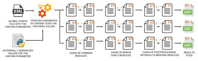
Figure 4-131 MC with a global parameter
