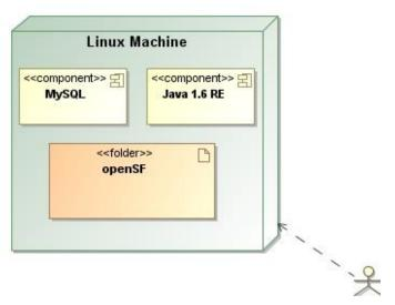
Figure 4-7 OpenSF deployment diagram
