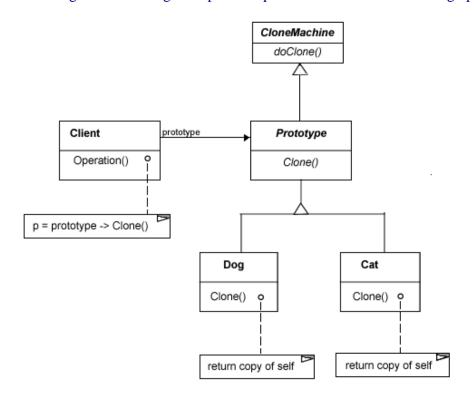
Figure 3-4 Prototype pattern example
