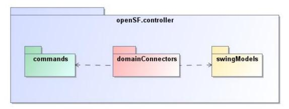
Figure 5-6: openSF.mmi.controller package diagram
