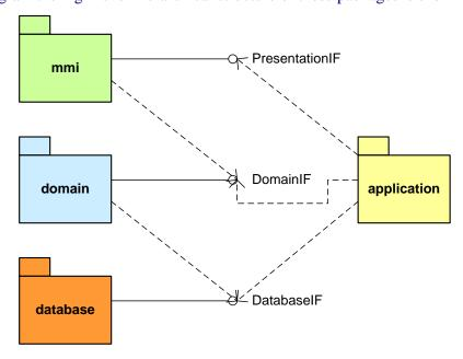
Figure 5-1: High-level package diagram
