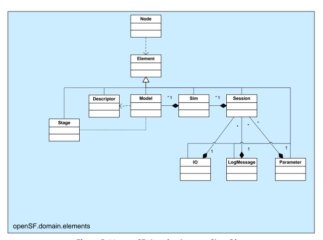
Figure 5-11: openSF.domain.elements Class Diagram
