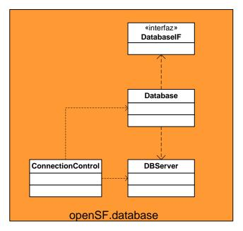
Figure 5-12: openSF.database class diagram
