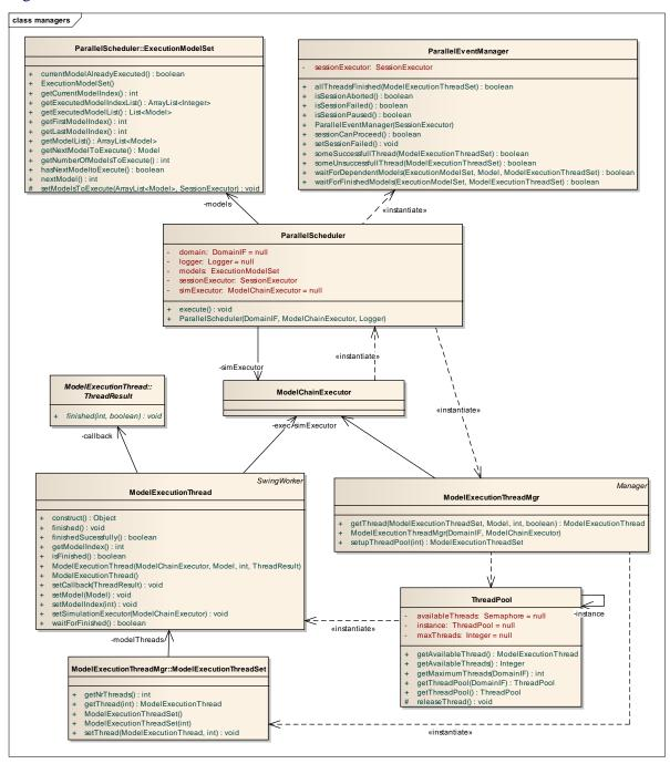
Figure 5-15: ModelChainExecutor class hierarchy for parallel model execution
