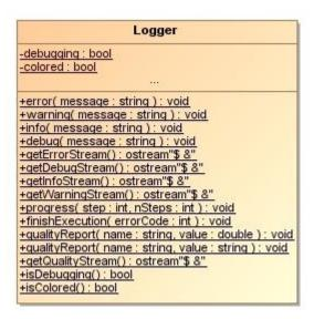
Figure 7-4: Logger class diagram
