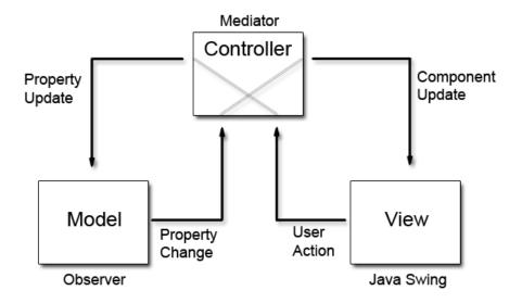
Figure 3-5: A simple diagram depicting the relationship between the Model, View, and Controller
