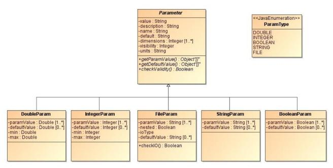
Figure 6-4: openSFpms.parameter class diagram
