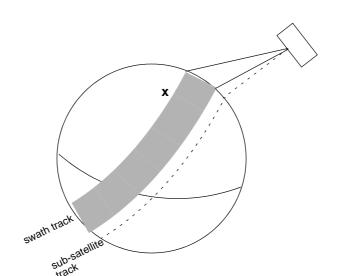
Figure 3 Earth-observing instrument: swath definition
