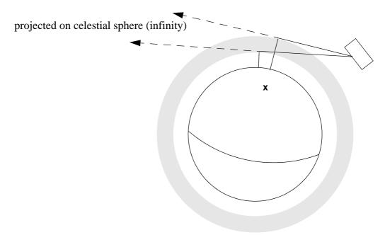
Figure 10 Two tangent altitudes over the ellipsoid
