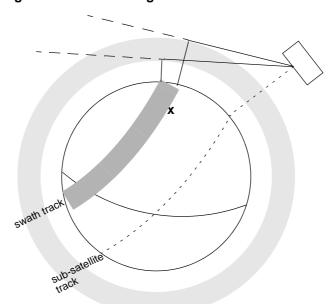
Figure 4 Limb-sounding instrument: swath definition (1)
