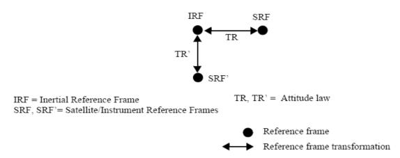
Figure 10: CFI-specific Reference Frames Transformations
