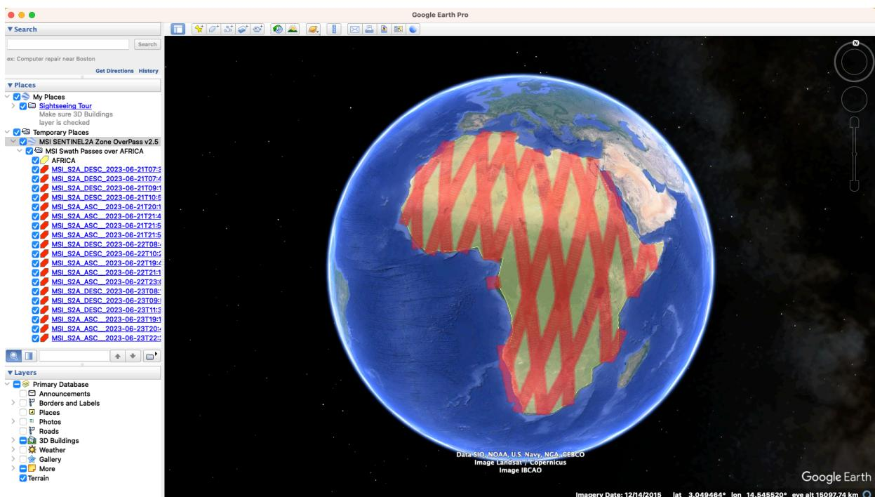
When moving the mouse over the swaths, the lines are highlighted (increase in thickness and lighter in colour). Then by clicking on top of the track, a balloon showing additional information is displayed, namely the absolute and relative orbit number sand the longitude and UTC time of the ascending node crossing of the selected orbit.
